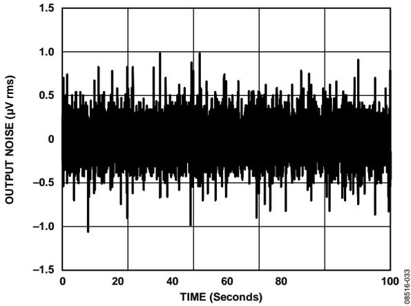
Figure 25. 0.1 Hz to 10 Hz Output Noise
