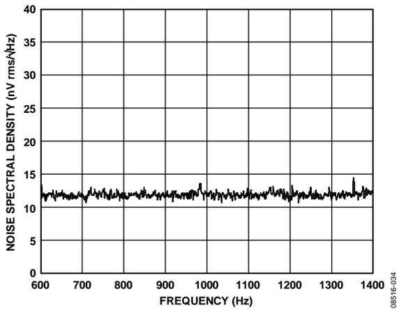
Figure 26. Noise Spectral Density vs. Frequency, 1 kHz
