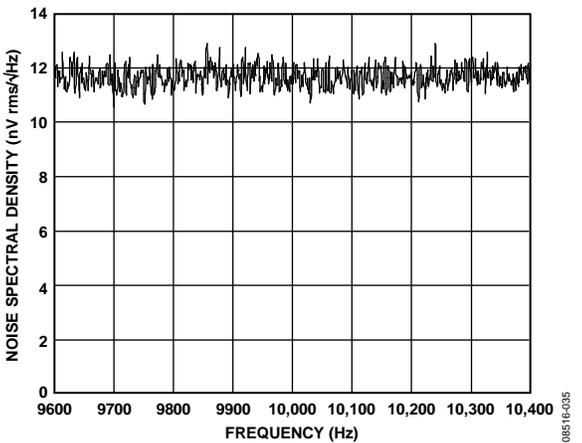
Figure 27. Noise Spectral Density vs. Frequency, 10 kHz
