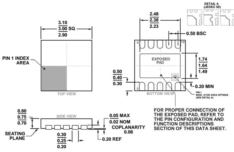
Figure 37. 10-Lead Lead Frame Chip Scale Package [LFCSP]
