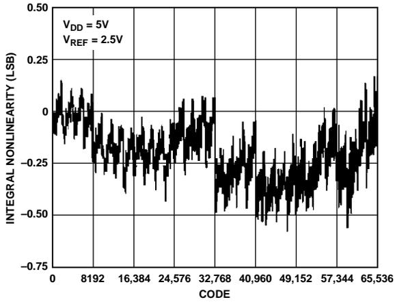
Figure 7. Integral Nonlinearity vs. Code
