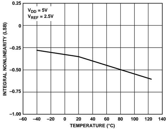
Figure 8. Integral Nonlinearity vs. Temperature
