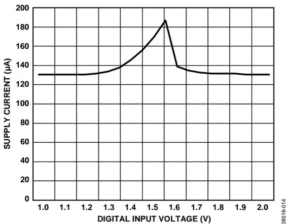
Figure 15. Supply Current vs. Digital Input Voltage
