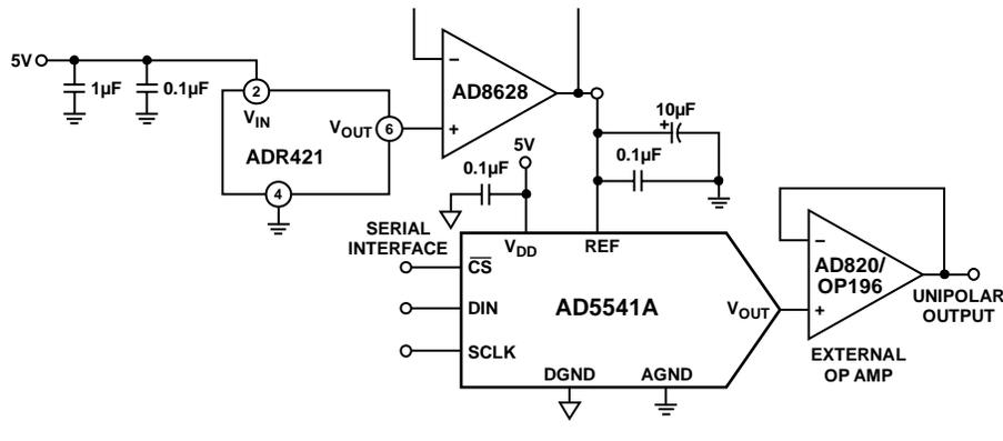
Figure 31. Unipolar Output
