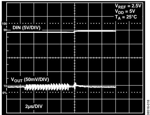
Figure 19. Digital Feedthrough
