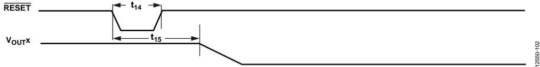
Figure 3. RESET Timing Diagram
