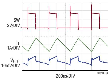
$3.3V_{IN}$  to  $1.2V_{OUT}$ , 2MHz TYPICAL APPLICATION
