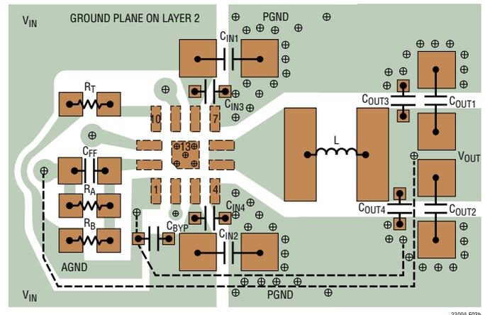
**Figure 3b. Recommended PCB Layout for the LTC3309A with capacitors  $C_{OUT1}$  and  $C_{OUT2}$  rotated by 90°, which reduces high-frequency output ripple. Optional 0201 capacitors  $C_{OUT3}$  and  $C_{OUT4}$  further improve the high-frequency output ripple**
