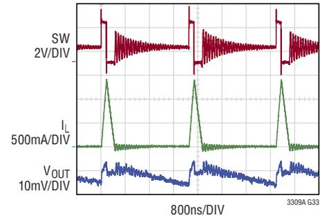
$3.3V_{IN}$  to  $1.2V_{OUT}$ , 2MHz TYPICAL APPLICATION
