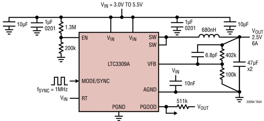
High Efficiency, 2MHz, 6A, 5V to 3.3V
