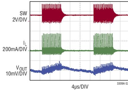
$3.3V_{IN}$  to  $1.2V_{OUT}$ , 2MHz TYPICAL APPLICATION
