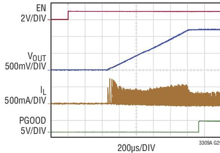
$3.3V_{IN}$  to  $1.2V_{OUT}$ , 2MHz TYPICAL APPLICATION
