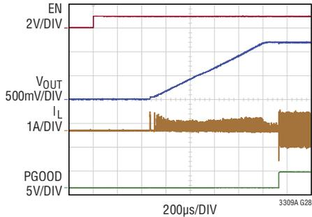
$3.3V_{IN}$  to  $1.2V_{OUT}$ , 2MHz TYPICAL APPLICATION
