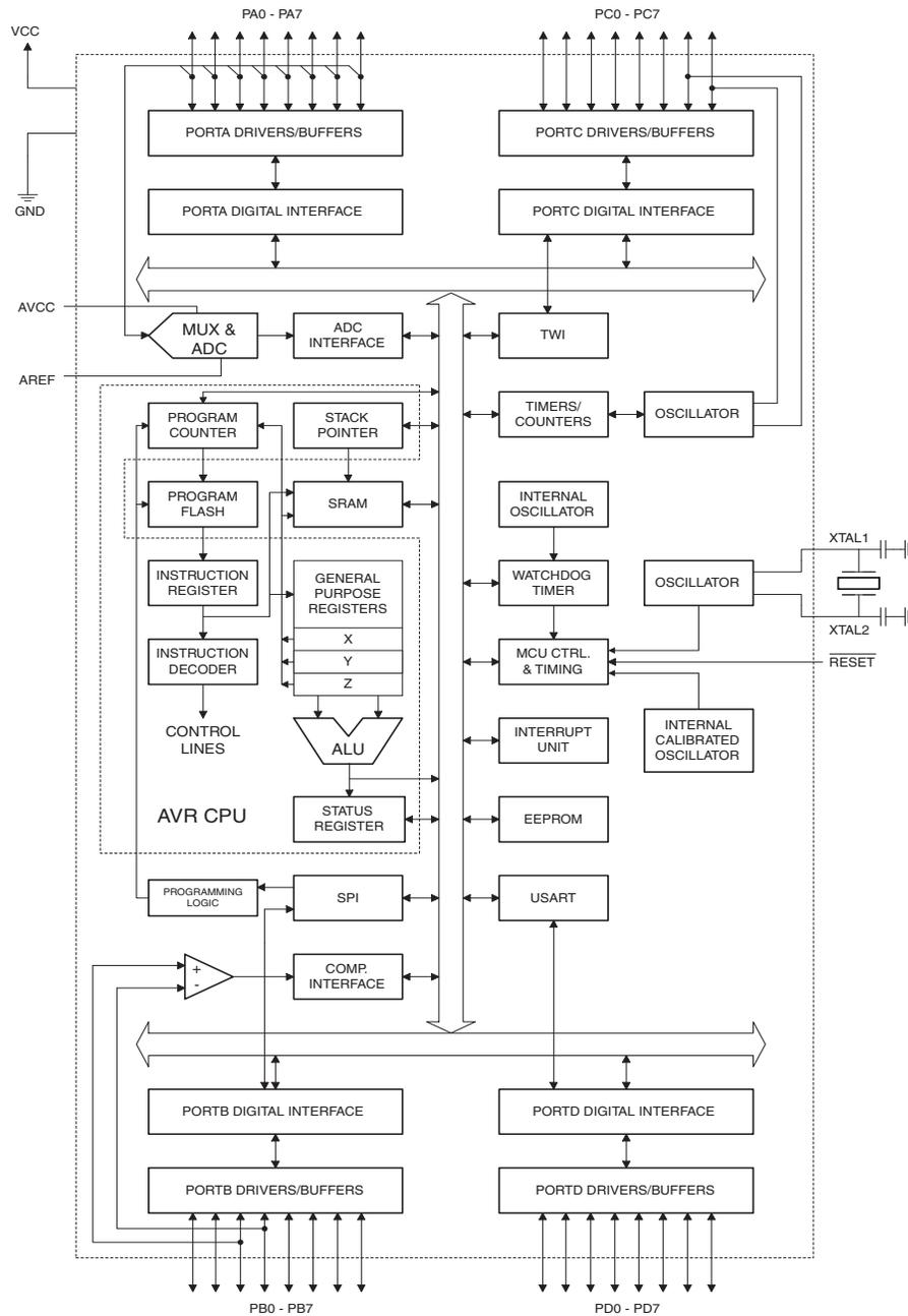
The Atmel®AVR® core combines a rich instruction set with 32 general purpose working registers. All the 32 registers are directly connected to the Arithmetic Logic Unit (ALU), allowing two independent registers to be accessed in
